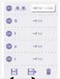
The stitches or text will be sequentially stored in the empty unit. Press the button (A) to save or press the button (b) to save and enter to combo sewing mode.
