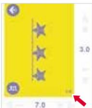
Then enter the combo sewing mode, the screen shows the stitch of the 1st combo position, on right bottom side appears current pattern/ total pattern. Press the start/stop button or step on the foot controller to start the sewing.
